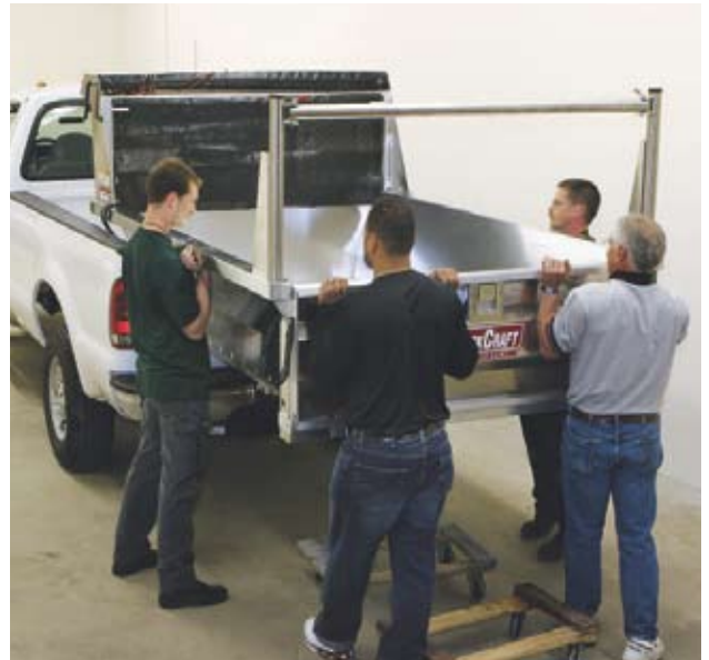
While many dump-bed inserts require the use of a forklift or winch, four able-bodied guys hoisted the lightweight aluminum dump-bed insert into the pickup without much fanfare. They placed pieces of carpet between the insert and pickup bed to prevent scratches.
