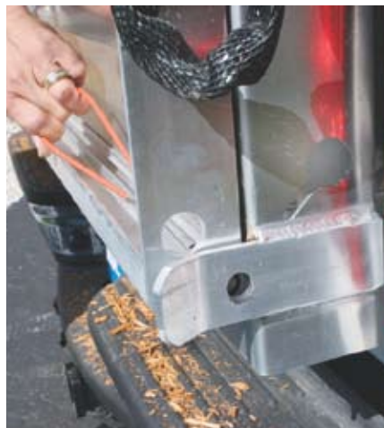
Dump beds usually have a dual-action tailgate that pivots either from the top or bottom so you can get rid of the material however you like. The tailgate can be removed from the dump insert by pulling the cables attached to spring-loaded lock pins.
