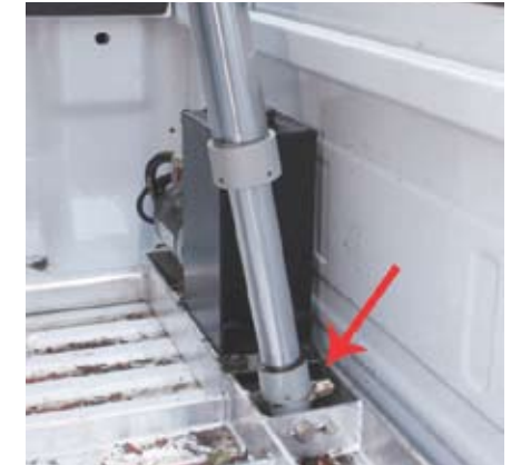
Allowing wood chips, rocks, and other debris to build up is the most common reason for premature hydraulic-ram problems. Keep the area around the ram free of these non-compressible items.
