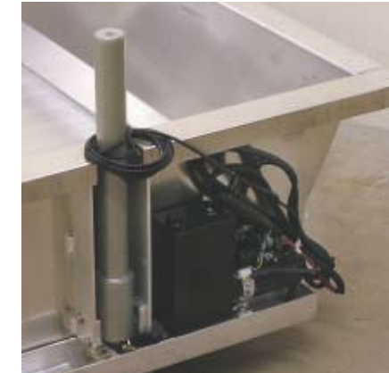
The real magic of these compact workhorses is the small yet powerful hydraulic pump and cylinder systems that lift the dump bed up. The TC-120 Ultra insert can lift 7000 pounds to 47 degrees in 18 seconds.
