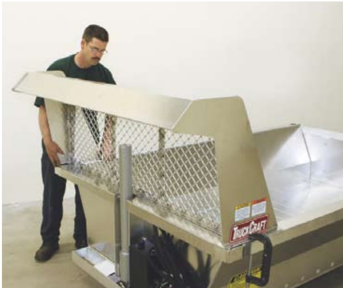
Weingartz Supply installed a SlipStream cab guard, a popular option for the TC-120 Ultra. The SlipStream protects the cab from the insert's contents, while its expanded metal grille ensures that the added safeguard doesn't reduce visibility.
